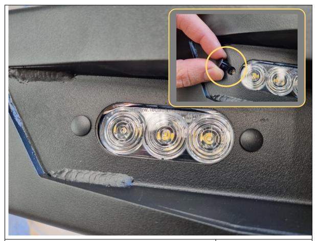
62. Plug the bolt access holes from the outside with the supplied black plastic hole plugs.
