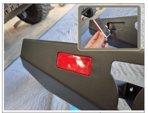
58. Remove the adhesive backing film from the supplied red retro reflectors and affix them to the opening on the outside of bumper wing. Press and hold firmly for 20 seconds. Do this for both wings.
