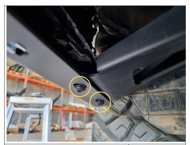
70. Also loosely secure the side of the wing to the wing brace with 2x M8x20 black button head bolts, washers and flange nuts.
