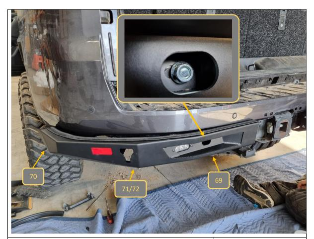
66. With assistance of another person, lift the wing up onto the vehicle. Ensure the M12 bolt fitted in the previous step fits through the slot shown.
