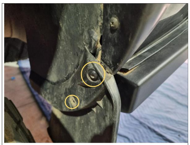
93. Refit the mudflap back to the bumper on both sides with the retained bolts and plastic push rivets.
