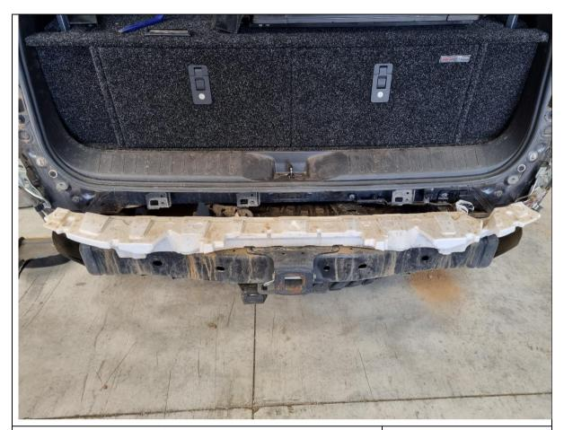
22. Remove the white foam step support and set aside.
