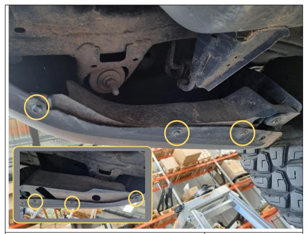
5. Remove 3x 10mm hex head bolts from the underside of the rear bumper on each side.
