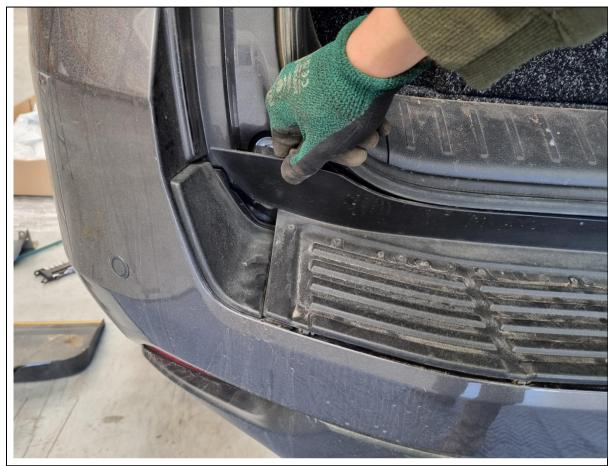
17. Starting from a top corner, pull upwards and outwards to remove the plastic tread panel. Set aside for later.
